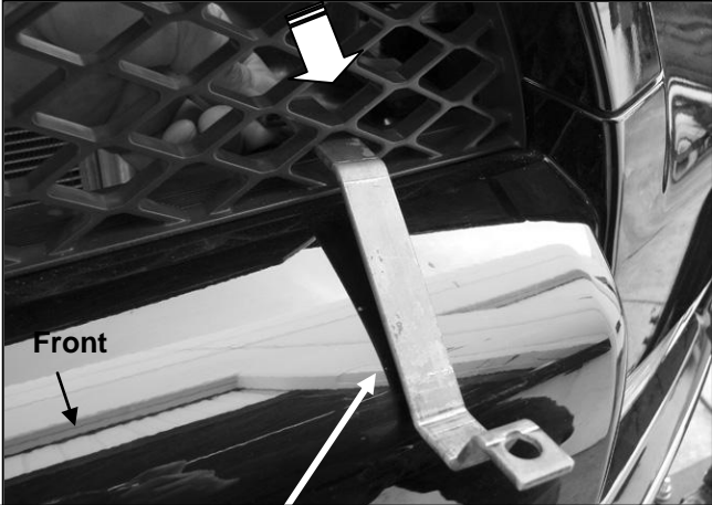
(Fig 11) 2010-13 models: Apply Adhesive Backed Foam Tape to the back of the Top Brackets to prevent damage to bumper cover during installation
