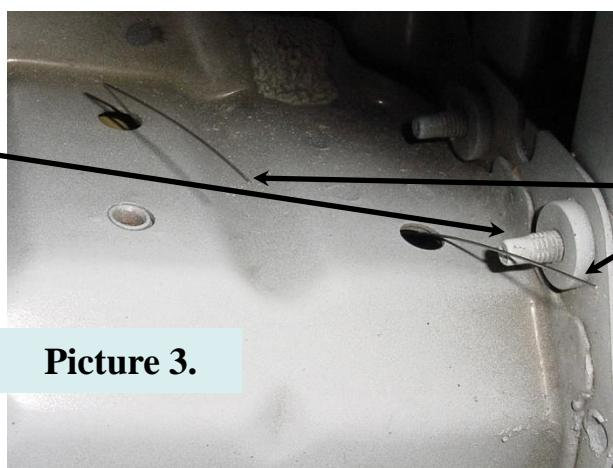
Slide hitch bracket up in place between outside of frame and inside of this bolt, typical both sides.
