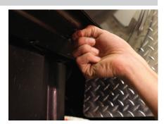
Insert the M10 bolt plate into the access hole in the rocker panel.
