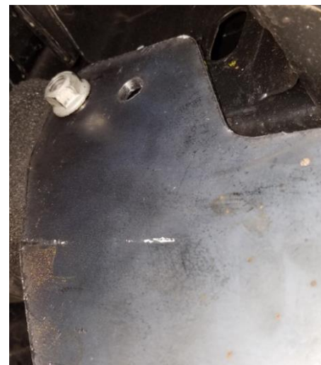
Driver side tow hook flange nut on flange bolt
