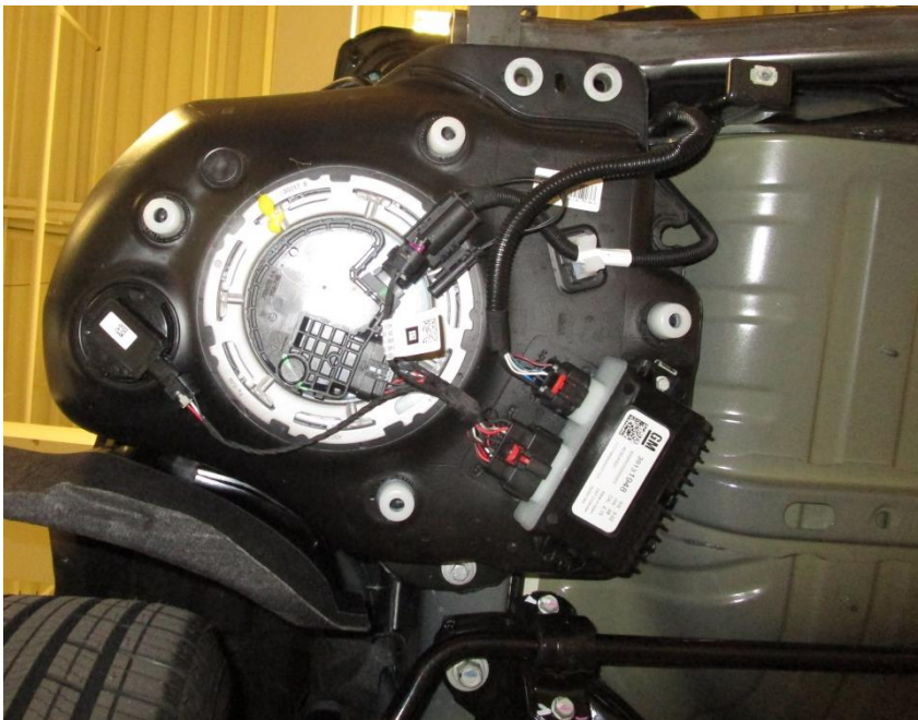
3 bolts, 3 electrical connections
