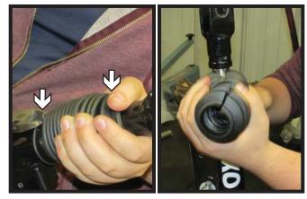
Remove the zipties securing the boot to the leg assembly. Remove the old boot.
