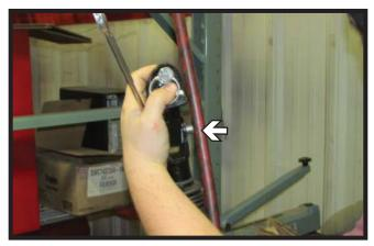
Using a 1/2" socket, remove the one (1) bolt attaching the lug to the leg assembly. Set the lug aside.
