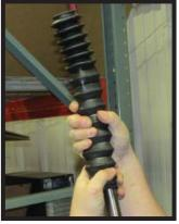
3. Coat the inside of the new boot with silicone spray, clean and regrease the leg assembly, and install the new boot.
