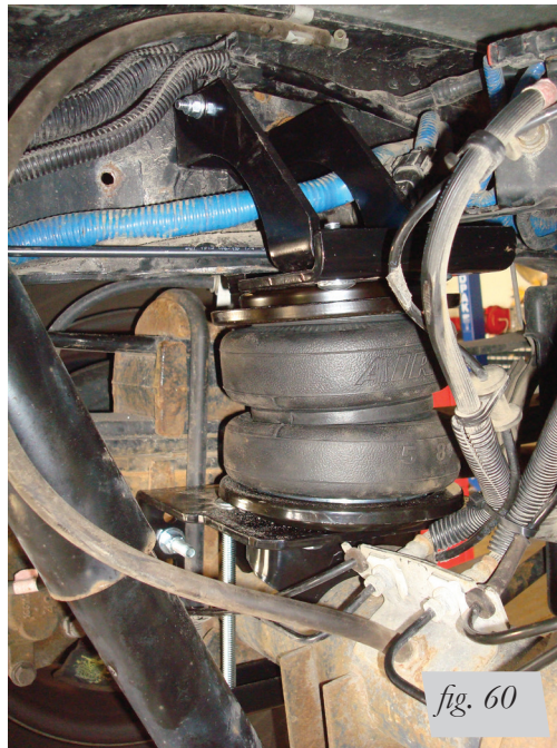
Left (driver's side) view of the kit installed from rear center of vehicle.
