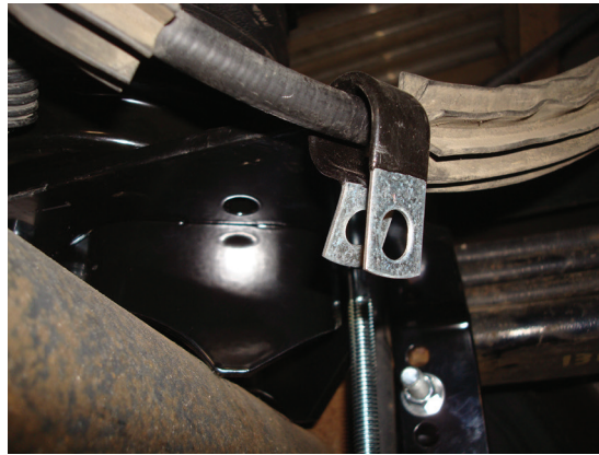
Set P-clamp over the emergency brake cable.
