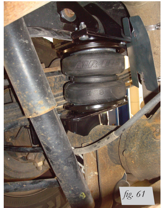
Right (passenger's side) view of the kit installed from forward of the axle.
