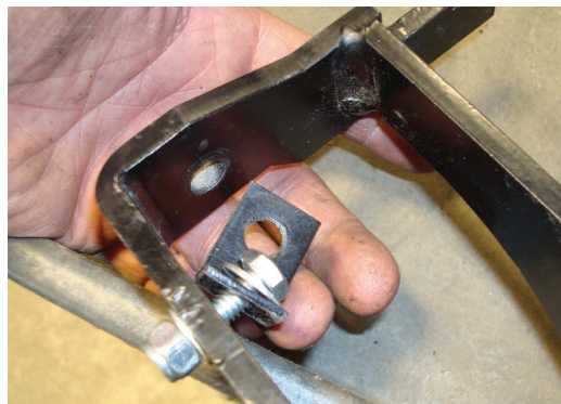
Attach the L-bracket to the brace in the position previously found using the hardware specified.
