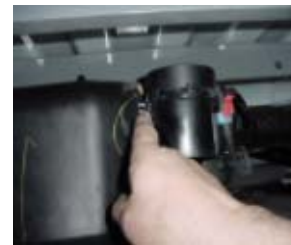
Figure C2, Step 2: Disengage the locking pin.
