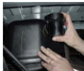
Figure C3, Step 3: Slide fuel valve from bracket.
