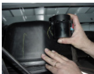
Step 3: Slide fuel valve from bracket.
