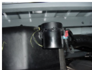
Step 1: Locate the fuel valve.
