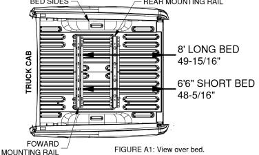
**IMPORTANT:** The mounting rail is designed to install only at the described location. Failure to place the mounting rail precisely may result in added difficulty during installation and/or property damage.
