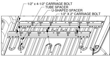
FIGURE C2: View looking down into the bed of the truck.
