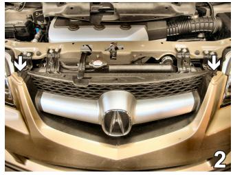
Between the headlight and the grille, on the top side of the fascia, remove two pushpins. Set pushpins aside.
