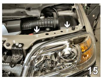
15. Using a 10MM socket. Pull the headlight assemblies forward to remove. Disconnect electrical connections. Set bolts and headlight assemblies aside to reinstall later.
