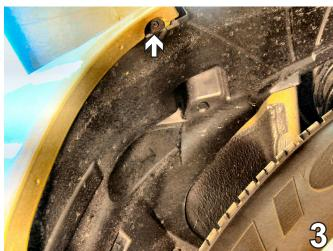
3. Just forward of the front tire, on the edge of the fascia, use an 8MM socket or Phillips screwdriver to remove one metric bolt. Set bolt aside to reinstall later. Do this to both sides of the vehicle.
