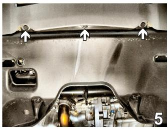
5. Remove three pushpins that run horizontally along the bottom of fascia, where the belly pan and fascia meet. Set bolts aside to be reinstalled later.
