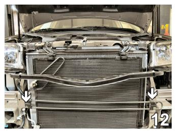
12. On the lower section of the radiator support, use a 10MM socket to remove the metric bolt of the coolant tubing bracket. Do this to both sides of the vehicle. Swivel the coolant line out of the way to clear the area for baseplate installation.
