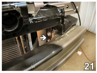
21. Tighten the bolts on the lower portion of the baseplate and all installed bolts in the top of the frame. Do this to both sides of the vehicle.
