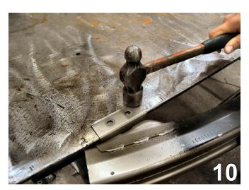
10. Lay the bracket of the metal bumper on a solid surface. Use a hammer to pound and flatten the rib on top of the bracket. Do this to both sides of the vehicle.
