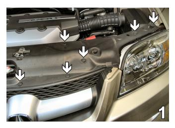
1. Remove 11 pushpins from the plastic above the radiator. Remove the plastic from the top of the radiator. Set pushpins aside to reinstall later.
