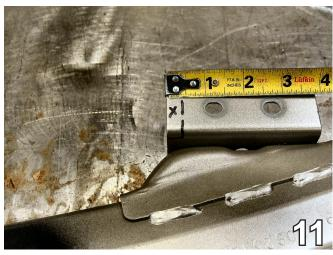
11. Mark and cut a section of the bumper bracket edge that faces toward the center of the bumper. Using the reciprocating saw, make a horizontal cut on the top of the bracket removing 3/8" from the end of the bracket. The cut travels the length of the top of bracket and down over the bracket lip about 1/4".
