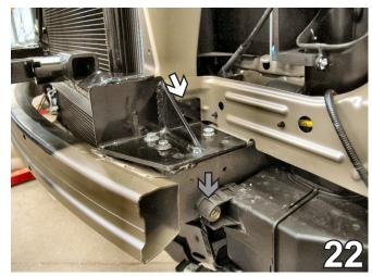
22. Align the nut plate with the drilled hole on the back side of the radiator support and tighten the 3/8-16 hex bolt and lock washer, as indicated by the white arrow in the photo. Do this to both sides of the vehicle. Using the 10MM socket, remove the metric bolt from the air baffle, as indicated by the grey arrow in the photo, and pull the air baffle down away from the frame.
