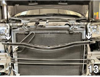
13. Using a 10MM socket, remove a metric bolt from either end of the headlight assemblies bracket. Set the bracket aside to be reinstalled later.
