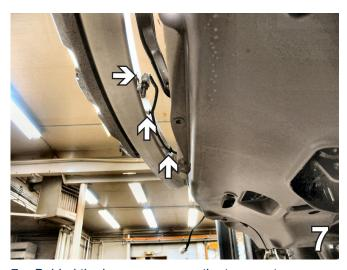
7. Behind the bumper, remove the temperature sensor from its clip. Also remove two pushpin connectors for the coax cable that are secured behind the bumper. Set temperature sensor and coax cable out of the way to be reinstalled later.
