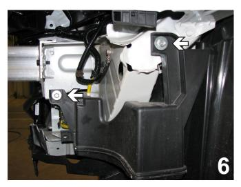
6. On the driver's side, remove the air baffle. Use a 10MM socket to remove the two metric bolts holding it. Set bolts aside to reinstall later.
