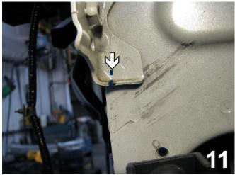
11. On the brace ridge make a cut, then flatten the side down. Do this to both sides of the vehicle.
