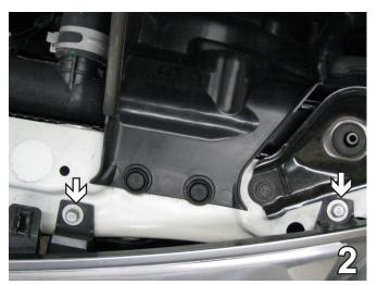
2. On the top side of the fascia, remove two metric bolts with a 10MM socket. Do this on both sides of the vehicle. Set bolts aside to reinstall later.
