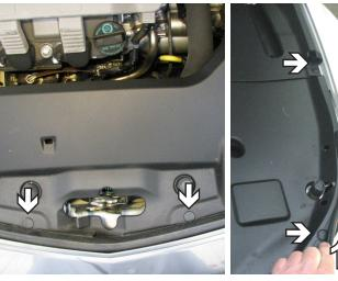
Remove six push pins from the plastic above the radiator, three on each side. Remove the plastic from the top of the radiator. Set pushpins aside to reinstall later.
