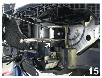
15. Slide the baseplate straight on. Align with the existing lower hole for air baffle on driver's side (gray arrow). Be sure the baseplate is level and clamp with a vise grip. The two lower baseplate holes should align to the middle of doubled lower frame webbing. Using the baseplate as a template, drill the four holes with a 13/32" drill bit. Do this to both sides of the vehicle.
