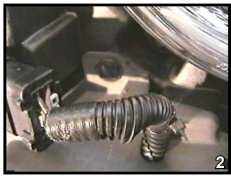
Remove the six push pins from the top side of the fascia. Disconnect the electrical plug on the driver's side as seen in the photo above.
