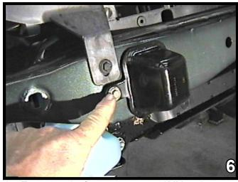
To remove the frame cup, use a 10MM socket to remove the metric bolt. Set cup and bolt aside to be reinstalled later. Do this to both sides of the vehicle. Some models may have tow hooks that will be removed at this time.
