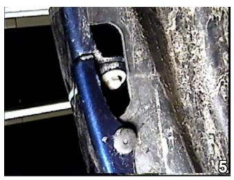
5. Using the 10MM socket, remove one metric bolt from the fascia's corner inside the wheel well. Set the bolt aside to be reinstalled later. Do this to both sides of the vehicle. Pull the fascia forward and set aside to be reinstalled later.
