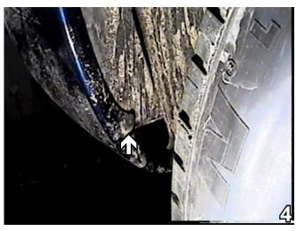
Just forward of the front tire, are two plastic rivets to remove using the diagonal cutters. These rivets will be replaced later with new (see the parts list).
