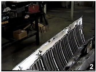
2. Pull the fascia forward and lift up to remove. Set the fascia aside to be reinstalled later.
