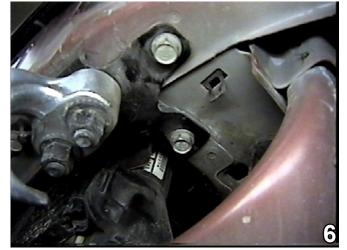
Using a 15MM socket, remove the factory tow hooks. Do this to both sides of the vehicle. The factory tow hooks will not be reinstalled later.
