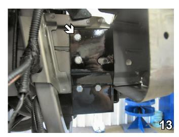
13. Insert the two (2) nut plates into the end of the frame rail to align with the top two (2) drilled holes, tighten the 3/8"-16 hex bolt and lock washer with the 9/16" socket. Do this to both sides of the vehicle.
