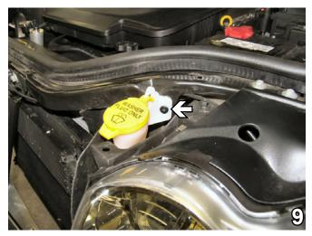
Remove a rivet from the reservoir spout with the diagonal cutters, pull reservoir down and set aside to be reinstalled later.
