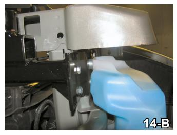
14. Align washer reservoir to its original position and install the existing backing bolt. Insert the 6MM-1.00 x 45MM hex bolt, 1/4" lock washer into the front washer reservoir bolt location, slide six (6) 3/8" flat washers between reservoir and baseplate, tighten to its original position (do **not** over tighten).
