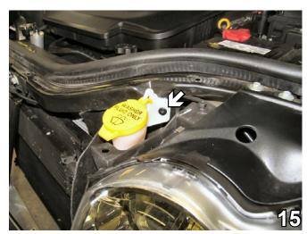
15. Tighten the 1/4"-20 x 3/4" bolt and flat washer into the existing bolt hole of upper reservoir spout. Tighten the 1/4" lock washer and hex nut on to the back side of the radiator support.
