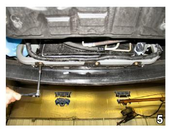
Using the 10MM socket, remove three (3) metric bolts from the lower radiator cross member.
