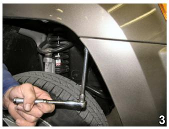
3. Using a 7MM socket, remove one (1) metric bolt from just forward of the front tire, on the fascia's corner. Do this to both sides of the vehicle. Set the bolts aside to be reinstalled later.
