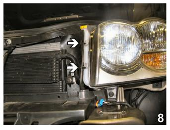
8. Remove two (2) christmas tree pushpins from the washer reservoir spout and air dam just inside of the headlight assembly on the driver's side.
