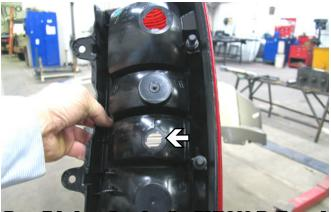
Possible location for the BX8869 Bulb and Socket Wiring Kit
