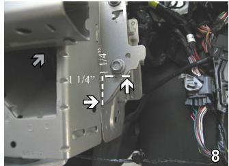
Using a reciprocating saw, notch out the corner by measuring up from the bottom 1 1/4" and 1 1/4" across. Do this on both sides. We recommend painting the cut edges to prevent them from rusting.
