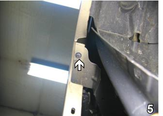
5. In front of the tire pull the wheel well cover back to remove the bolt with a 7MM socket. Do this on both sides. Set the bolt aside to be reinstalled later. Pull forward on the fascia to remove it, disconnect the turn signals and running lights (if applicable). Do this on both sides. Set the fascia aside carefully to be reinstalled later.
