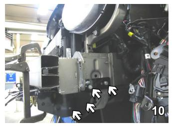
10. On the driver's side, insure the baseplate is level with the frame and clamp in place with the large vice grips. Using the baseplate as a template, drill four holes into the frame with the 13/32" drill bit.
