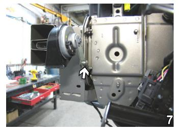
7. Use a 10MM socket on the back to remove the bolt and horn. Set aside to be reinstalled later.
