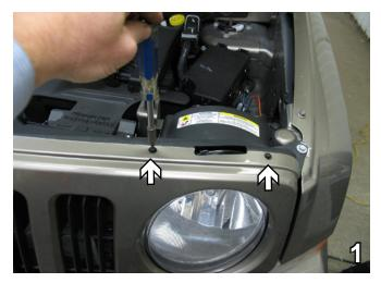
1. Remove seven bolts with a T20 Torx from across the top of the fascia (driver's side shown in photo). Set bolts aside to be reinstalled later.
