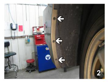
Just forward of the front tire, inside the wheel well, remove three bolts with a 7MM socket. Do this to both sides of the vehicle. Set bolts aside to be reinstalled later.
