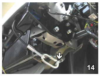
14. Attach the permanent baseplate safety cables to the provided convenience link on the baseplate. The photo above shows the recommended installation of the cables to frame of vehicle. Additional options may interfere with suggested mounting; in this case secure the cables to a solid piece of the frame as described in the instructions included with the permanent baseplate safety cables. Be sure the safety cables do not rub against any hoses or moving parts. Do this to both sides of the vehicle.
