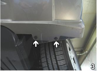
3. Under the fascia remove the two pushpins in front of the tire. Do this to both sides of vehicle. Set pushpins aside to be reinstalled later.
