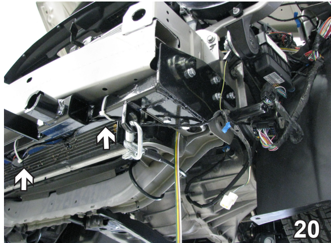
20. Zip tie the sensor to the bottom of the baseplate and reconnect.
