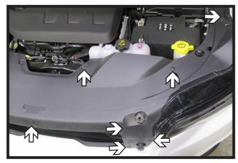
Remove the thirteen (13) push pins from the fascia cover. There are six (6) on each side and one (1) in the center. Remove fascia cover and set aside to be reinstalled later.
