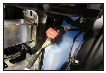
7. As the fascia is removed unhook the plug on the driver side by pulling out the yellow piece and up on the red part to unhook. Remove fascia and set aside to be reinstalled later.
