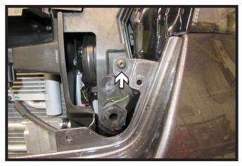
Using a T30 Torx, remove the two (2) bolts from the fascia, there is one (1) on each side.
