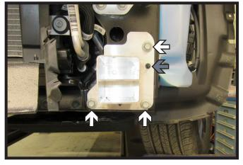
Using a 15MM socket, remove the three
