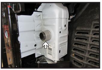
Using an extra large crescent wrench, remove the nut from the driver side of the vehicle. Slide tube back and out of the way to be reinstalled later.
