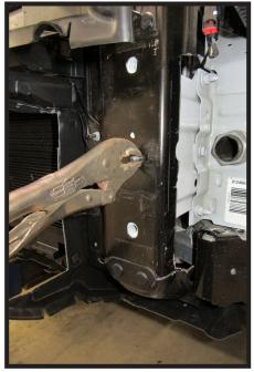
Using vice grip pliers, shake bolt to loosen. Then using a hammer, pound out bolt and remove. Do this on both sides of vehicle.
