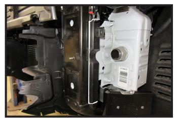
11. Using a reciprocating saw, trim the frame as indicated. Do this on both sides of the vehicle.
