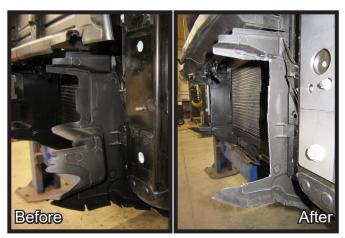
12. Using a utility knife, cut and remove the area from plastic shroud as shown. Do this on both sides of the vehicle.
