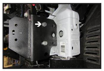
Insert spacer plate at top of baseplate between the frame and baseplate with the slotted end facing downward. Once spacer plate is in position insert 1/2" x 1-1/2" bolt with lock washer and whiz nut into top front hole.
