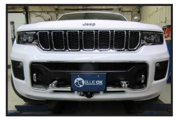
22. Hold the fascia as close to its original position, mark and trim the fascia around the convenience links and attachment tabs. Reinstall the fascia, fascia cover, belly pan and reconnect all electrical connections.
