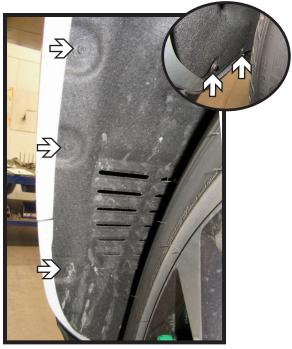
Using an 8MM socket, remove the five (5) bolts from along the edge of wheel well. Do this on both sides of the vehicle.
