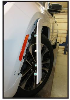
6. Unsnap the wheel well trim just past fascia joint. Hold trim away from fascia using a soft cloth. Do this on both sides of the vehicle.
