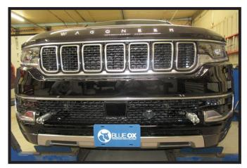
17. Hold the fascia as close to its original position, mark and trim the fascia around the convenience links and attachment tabs. Reinstall the fascia.
