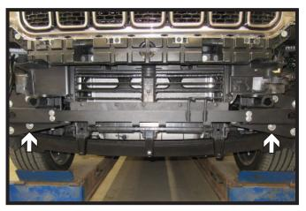
14. Install two (2) 1/2" x 1-1/2" bolts with flat washers and nylon lock nuts into the bottom inside of the holes on the front of the vehicle.
