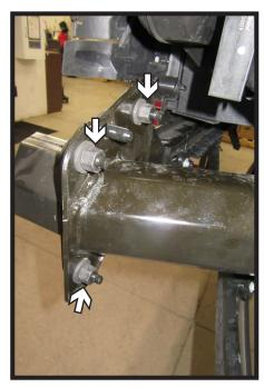
Using a 18MM socket or wrench, remove the four (4) nuts from the bumper on the driver side and three (3) nuts from the passenger side. Remove bumper, it will not be reinstalled.
