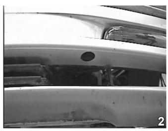
Remove the #12 Torx bolts from below the headlight. Do this on both sides of the vehicle. Set bolts aside to be reinstalled later. Unplug the running lights, and pull the fascia forward from the vehicle. Set the fascia carefully aside to be reinstalled later.
