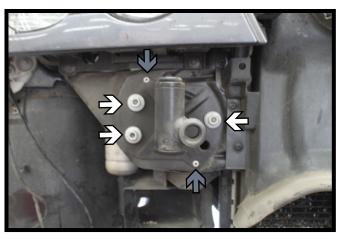
5. Using a 13MM socket, remove the three (3) nuts from the bumper support (white). Then drill out the two (2) rivets (gray). Do this on both sides of the vehicle.
