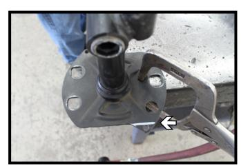
8. On the bumper support, trim off the lower tab. Do this on both supports.
