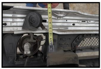
13. On the backside of the fascia, measure down from the top of the fascia approximately 7". Mark and trim an area 1" wide x 1-1/4"high for baseplate clearance.
