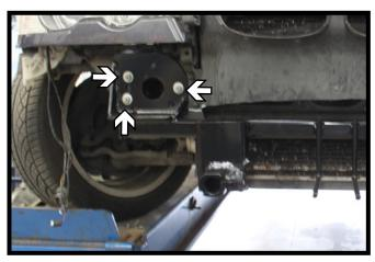
Attach the baseplate to the vehicle using the existing nuts. Do this on both sides of the vehicle.
