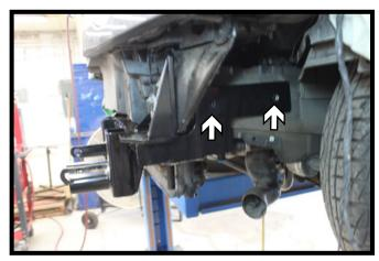
10. Using a 13/32" drill bit, drill the two (2) holes in the side of the baseplate thru the frame. Install 3/8"-16 x 1-1/2" bolts with 3/8" lock washers into the holes and 3/8"-16 nut plates on the inside of the frame. Do this on both sides of the vehicle. Fully tighten all fasteners.
