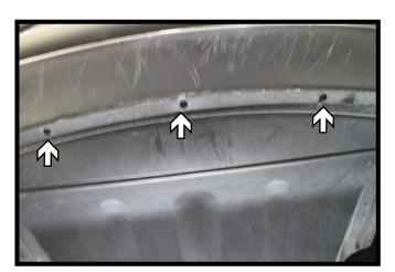
3. Remove the three (3) push pins from the underside of the fascia.
