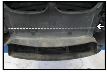
Trim the air dam off just below the bolt heads across to allow baseplate clearance.
