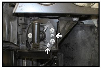
11. Remove the nuts installed previously from step #9. Using a 13/32" drill bit, drill the outer two (2) holes of the baseplate thru the face of the frame. Transfer the hole locations to the support and drill out. Reinstall the support with the existing nuts and install 3/8"-16 x 1-1/2" bolts with 3/8" flat washers into the holes and 3/8" lock washer and nut on the backside of the face. Do this on both sides of the vehicle.
