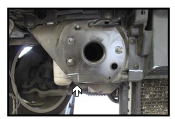
7. Using a reciprocating saw, trim a 1" x 1" notch out of the face of the frame. Do this on both sides of the vehicle.
