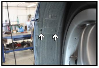
Using a 8MM socket, remove the two (2) screws from the wheel well. Do this on both sides of the vehicle.
