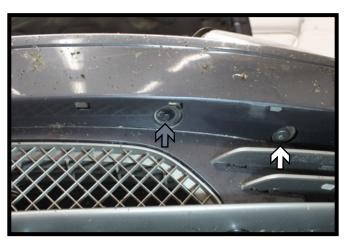
1. Using a T50 Torx, remove the screw from the underside of the bumper (white). Then remove the push pin (gray). Do this on both sides of the vehicle.
