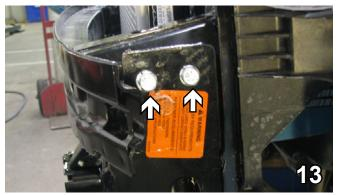
13. Into the holes drilled in the side also insert  $3/8-16 \times 1 1/4$ " bolts with Loctite, 3/8" lock washers and 3/8" nut plates. Do this on both sides.
