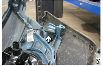
7. Located on both sides behind the grill, there is a temperature sensor that will need to be unplugged.
