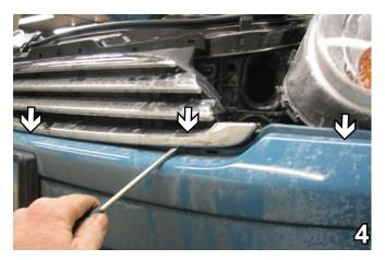
4. Remove the grille by starting from the side and working across. Use a screwdriver to pry and release the clips. They will fit back in when reinstallation occurs. Set the grille aside for later reinstallation.
