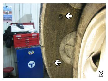
2. Forward the front tire, use a Phillips screwdriver to remove two pushpins. Do this to both sides. Set aside for later reinstallation.
