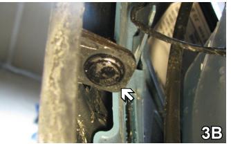
3. After removing the wheel well cover, remove two pushpins connecting the fascia using a flat screwdriver. Do this to both sides. Set pushpins aside for later reinstallation.
