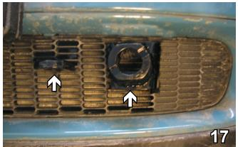
17. Reconnect the temperature sensor. Hold the fascia up to its original location. Mark and trim the fascia just on the outside edges of the receiver tube and convenience links. Do this to both sides of the vehicle. Reinstall the grille.
