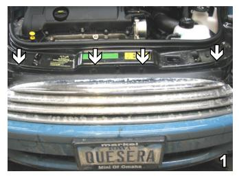
1. Using a flat screwdriver, remove four pushpins on top edge of grille, one on each side two in the middle. Set push pins aside to be reinstalled later.
