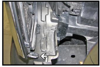
Reach down underneath the corner of the headlight, push down on the clip on the corner of the grille and pull to release. Do this on both sides of the vehicle.
