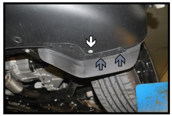
7. Using a T25 Torx, remove the screw from the underside of the fascia (white). Then the two (2) push pins next to the screw (gray). Do this on both sides of the vehicle.
