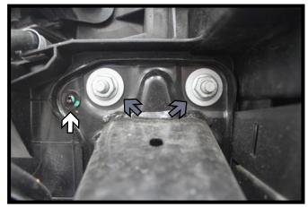
12. Using a T20 Torx, remove the screw from the top side of the bumper (white). Then using a 16MM socket, remove the two (2) nuts (gray). Do this on both sides of the vehicle.
