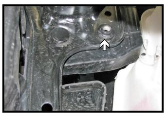
13. Using a 16MM socket, remove the bolt from the backside of the middle bumper bracket. Do this on both sides of the vehicle.
