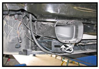
22. Reinstall the brake duct baffles on both sides of the vehicle.
