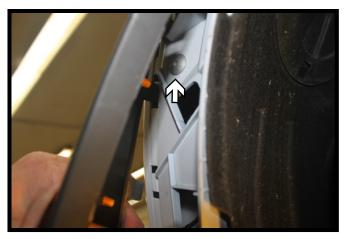
6. Unsnap the fender flare from the body. Behind the flare, using a T25 Torx, remove the screw from the fascia. Do this on both sides of the vehicle.
