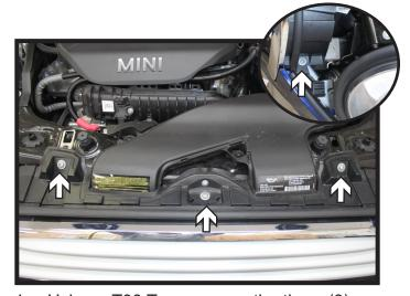
Using a T30 Torx, remove the three (3) screws from the top edge of the fascia. Then remove the two (2) screws next to the headlights, there is one (1) on each side (inset).
