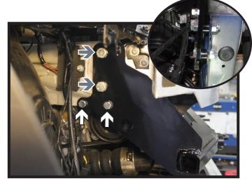
Install the baseplate to the vehicle using the existing frame holes with the supplied 12MM bolts and lock washers (gray). Level and fully tighten all bolts.
