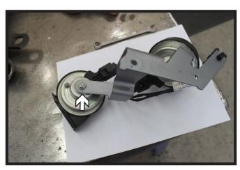
13. Using a 10MM socket, remove the screw from the lower horn.
