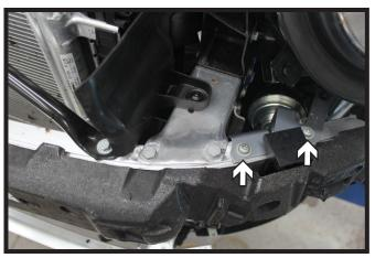
6. On the driver side, using a T30 Torx, remove the two (2) screws from the horn bracket. Disconnect all lines and set the horn assembly aside.
