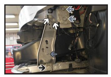
7. Using a T30 Torx, remove the two (2) screws from the top of the support bracket (white). Using a T25 Torx, remove the screw from the duct (gray). Using a 8MM socket, remove the bolt from the bottom of the support bracket (black).
