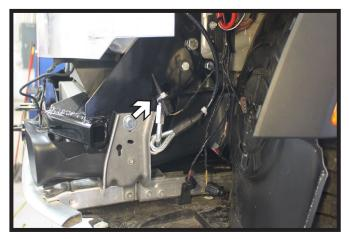
On the driver side, ziptie the temperature sensor securely.
