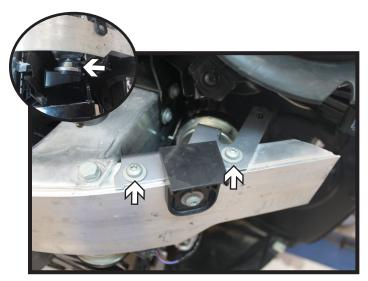
Leaving the lower horn loose, reinstall the bracket to the vehicle. After the bracket is reinstalled reattach the lower horn to the bracket.
