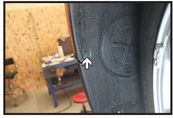
Using a 8MM socket, remove the screw from the outer edge of the wheel well. Do this on both sides of the vehicle.
