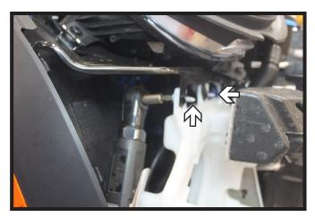
Using a T30 Torx, remove the two (2) screws from the washer reservoir.
