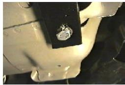
8. Drill a 13/32" holes using the lower bracket as a template on both sides. Insert items 3, 5, and 6 according to drawing on last page. Be sure and use loctite on all bolts before tigthening.
