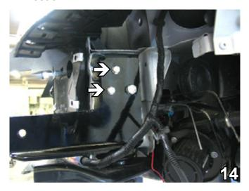
14. Using the endplate as a template, drill two holes into the frame with the 13/32" drill bit. Insert 3/8"-16 nut plates into frame rail opening and align to drilled holes. Insert 3/8"-16 x 2-1/2" bolts and 3/8" lock washers into holes and tighten. Do this to both sides of the vehicle.
