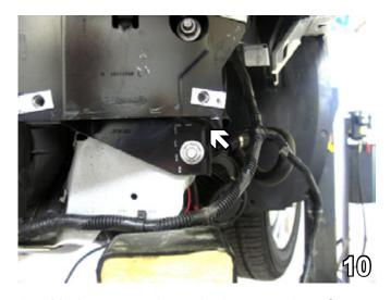
10. Mark a rectangle on the lower portion of bumper bracket. Start horizontally below the upper portion of bumper bracket (see white arrow) and continue just beyond the lower bolt hole. Then, mark straight down until reaching bottom of frame rail. This vertical marking should be flush with frame rail edge (behind bumper bracket). Using the reciprocating saw, cut marked area through the bumper bracket and frame rail.
