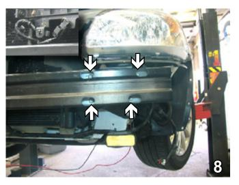
8. Under hood latch area (see inset), disconnect two (2) electrical connections and move out of the way. Using the 13mm socket, remove four (4) metric bolts from the metal bumper. Do this to both sides of the vehicle. Set bolts aside to be reinstalled later.
