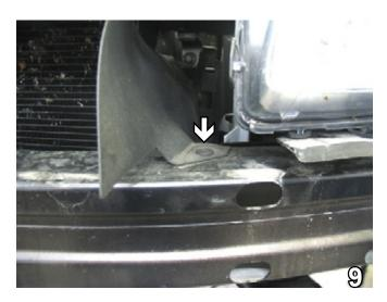
Remove one (1) pushpin fastening the lower section of air dam to the top of the metal bumper. Do this to both sides of the vehicle. Pull metal bumper forward to remove. Set pushpins and metal bumper aside to be reinstalled later.
