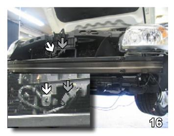
16. When reinstalling electrical connections under hood latch area, the tab-style connector goes to it's original location (see grey arrow). Snap the other connector into place (see white arrow), entering from the backside of it's bracket (rather than from the front).
