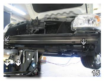
15. Place cross tube between the endplates (see grey arrows). Insert 1/2"-13 x 1-1/4" bolts into the endplate's two (2) front holes (see white arrows of inset). Tighten the forward most bolt and 1/2" lock washer to the weld nut in the cross tube. Tighten the other front bolt to the 1/2" lock washer and 1/2"-13 hex nut. Do this to both sides of the vehicle.
