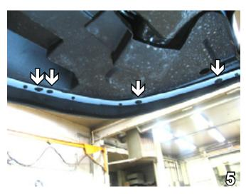
Remove four (4) pushpins from the bottom corner of fascia. Do this to both sides of the vehicle. Set pushpins aside to be reinstalled later.
