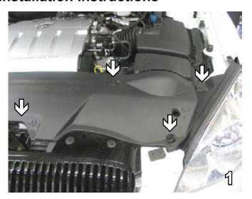
Remove four (4) pushpins from the radiator cover and lift to remove. Do this to both sides of the vehicle. Set pushpins and radiator cover aside to be reinstalled later.
