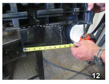
12. Remove the fascia support from the back of the fascia. Using the utility knife, start a vertical cut 7-1/2" in from the fascia support's inside edge. Cut upward until stopped by molding. Then, cut horizontally until reaching the inside edge. Do this to both sides of the vehicle. Reinstall fascia support to the back of fascia.
