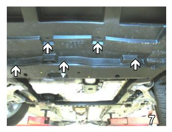
7. Remove five (5) pushpins from the belly pan. Set pushpins and belly pan aside to be reinstalled later.
