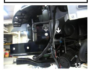
13. Align endplate with existing hole of the frame rail. Insure top of endplate is parallel with frame rail. Insert 1/2"-13 nut plate into frame rail opening (see white arrow) and align to pre-existing hole. Insert 1/2"-13 x 2-1/2" bolt and 1/2" lock washer and tighten (see grey arrow). Do this to both sides of the vehicle.
