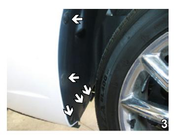
3. Remove five (5) pushpins just forward of the front tire, on the edge of fascia. Do this to both sides of the vehicle. Set pushpins aside to be reinstalled later.
