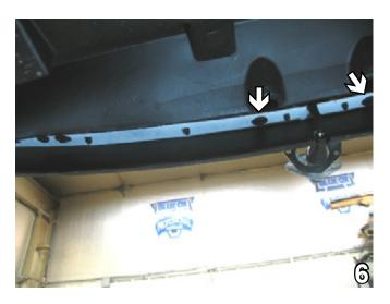
6. Remove two (2) pushpins from the bottom center of fascia. Pull fascia forward to remove. Set pushpins and fascia aside carefully to be reinstalled later.
