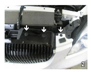
2. Remove three (3) pushpins from the top of the fascia. Do this to both sides of the vehicle. Set pushpins aside to be reinstalled later.
