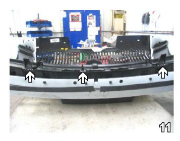
11. Using the utility knife, remove three (3) tabs from the lower edge of fascia support. *Note:*To prevent scratching, fascia should be lying on a smooth surface.
