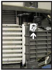
14. If needed use a reciprocating saw to trim the indicated areas on both sides of the vehicle so that they are flush with the frame.
