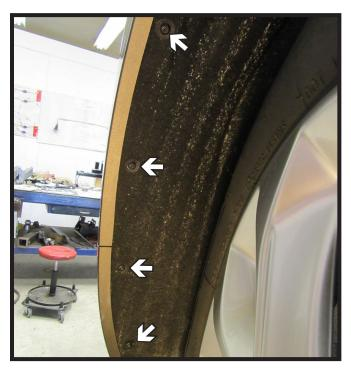
Using a T15 Torx socket, remove the four (4) bolts from the wheel well liner. Do this on both sides of the vehicle.
