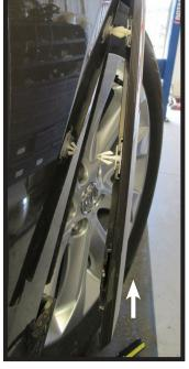
4. Pull back the wheel well liner. Using a 7MM socket remove the bolt (gray arrow). Then release the clips from the fender flare (left, white arrow). Pull straight up on the flare to release the bottom and then out away from the vehicle. Do this on both sides of the vehicle.
