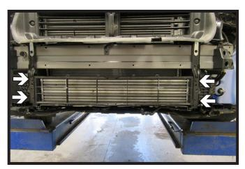
Using a T25 Torx socket, remove the four (4) bolts from the lower grille and set it aside. It will not be reinstalled.
