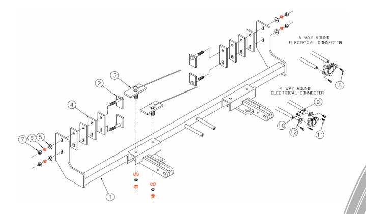
**IMPORTANT:** Use only genuine factory replacement parts on your Base Plate. Do not substitute homemade or nontypical parts. If a bolt is lost or in need of replacement, for your safety and the preservation of your Base Plate, be sure to use a replacement bolt of the same grade (Usually Grade 5, refer to parts list). Repair parts may be ordered through your nearest **Blue Ox** dealer or distributor.
