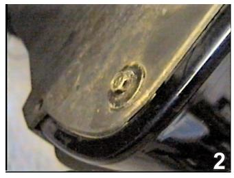
Using the 7MM socket, remove three metric bolts inside the wheel well. Do this to both sides of the vehicle
