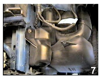
7. Remove the windshield washer reservoir using the 10MM socket on the three side bolts, one bolt on the bottom, with the 7MM socket and one Phillips screw on the outer tubing. Pull the reservoir down, disconnect the electrical connections, cap pump tube and set aside to be reinstalled later. Remove the horn bracket on the passenger's side of the vehicle with the 10MM socket.
