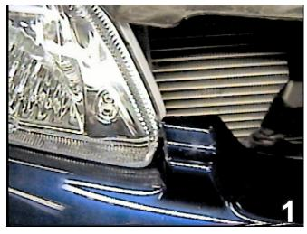
Remove four pushpins from the top side of the fascia. Set the pushpins aside to be reinstalled later.
