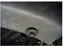
4. Remove seven push pins from the bottom of front fascia, unplug side lights. Pull fascia forward and set aside.
