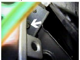
3. Using the 10MM socket, remove one metric bolt inside wheel well on upper fascia corner, both sides.
