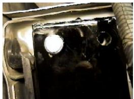
7. Drill remaining holes with the 13/32" drill bit. Install items 3, 4 and 5, tighten all bolts, both sides. Be sure and use loctite on all bolts before tightening. Tighten according to torque chart in the General Instruction Sheet.
