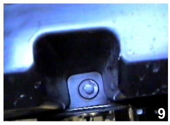
Remove one pushpin from the lower plastic on the bottom rib of the frame and pull plastic down to expose the bottom of the frame. Set pushpin aside to be reinstalled later. Do this to both sides of the vehicle.
