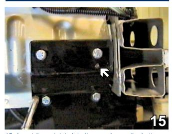
15. Insert the nutplate into the opening on the bottom of the frame to align with the upper drilled holes on the passenger's side, tighten the lock washer and the hex nut. Using the baseplate as a template, drill the hole on the passenger's side with the 1/4" drill bit (see the arrow in the photo above).
