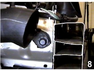
8. Remove two pushpins from the air baffle on the passenger's side and using a 10MM socket, one metric bolt behind the wheel well. Set pushpins and bolt aside to be reinstalled later.
