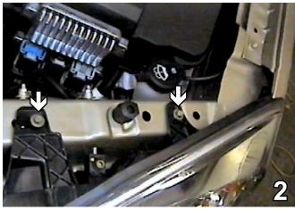
Using a 10MM socket, remove two metric bolts from the headlight assembly. Pull the headlight assembly forward, unplug the electrical connections. Set the headlight assembly and the metric bolts aside to be reinstalled later. Do this to both sides of the vehicle.
