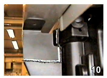
10. Using the utility knife, trim the air dam 2 1/2" below the metal bumper to open the area for the baseplate. Do this to both sides of the vehicle.
