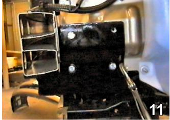
11. Align the upper back baseplate hole with the horn bracket mounting hole on the driver's side and clamp the baseplate in place with the vise grips. Measure driver's side height on frame and the distance from the back of metal bumper, clamp passenger's side to the same locations on the frame.
