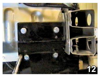
12. Using the baseplate as a template, drill the four holes on the passenger's side and three holes on the driver's side with the 13/32" drill bit.
