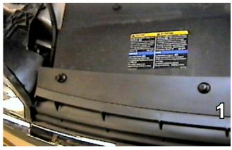
1. Remove the four Phillips head pushpins from the black plastic cover on the top side of the fascia. Set the pushpins aside to be reinstalled later.
