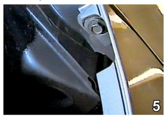
5. Using a 10MM socket, remove one metric bolt from just forward of the front tire, on the fascia's corner. Set the bolt aside to be reinstalled later. Do this to both sides of the vehicle.
