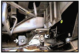
Using the 15MM socket, remove two
