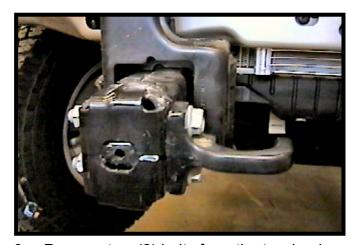
8. Remove two (2) bolts from the tow hook using the 18MM socket. Do this to both sides of the vehicle.
