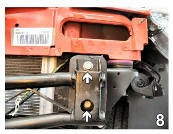
Using a 15MM socket, remove two metric bolts from the metal bumper. Do this to both sides of the vehicle. Pull metal bumper forward and set aside with the bolts to be reinstalled later.
