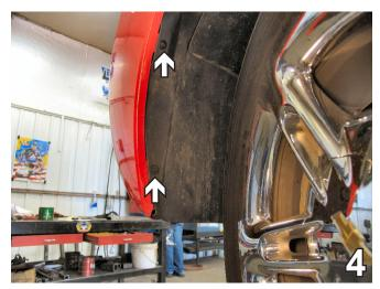
Using the 7MM socket, remove two metric bolts just forward of the front tire, inside the wheel well.
