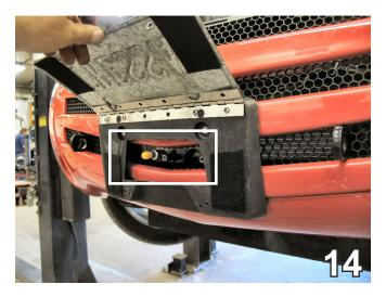
14. Adjust the electrical rods behind the license plate as needed to fit through the openings.
