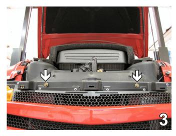
3. Using the 10MM socket remove 2 metric bolts from the top of the fascia.
