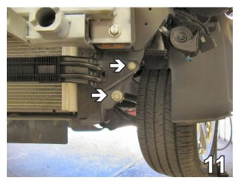
11. Using a 10MM socket, remove the bolt securing the coolant tubing. Do this to both sides of the vehicle. Remove the tubing and set aside to be reinstalled later. This will allow you to access the frame rail to install the shim plates.
