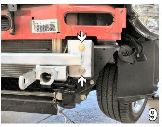
9. Align the baseplate so that it is flush with the top of the frame rail and slide completely to one side of the frame rail.
