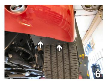
6. Remove two push pins on the lower edge of the fascia, just forward of the front tire. Do this to both sides of vehicle. Set push pins aside to be reinstalled later.
