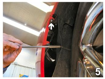
Pull wheel well cover back to expose one metric bolt. To be removed with a 10MM socket to remove it. Do this to both sides of the vehicle. Set bolts aside to be reinstalled later.
