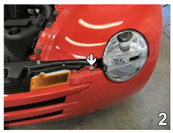
2. Using the 10MM socket, remove the nut next to the headlight assembly. Do this to both sides of the vehicle. Set nuts aside to be reinstalled later.
