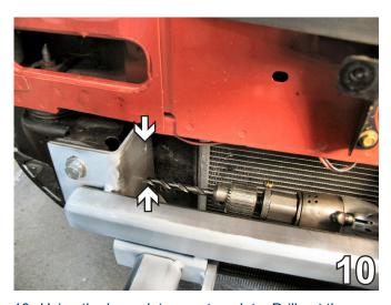
10. Using the baseplate as a template, Drill out the remaining tow holes in the side of the frame rail with the 13/32" drill bit. Insert the 3/8-16 nut plates through the bottom of the frame rail, behind the horn, and align with drilled holes. Install the 3/8-16 x 1 1/2" hex bolts and 3/8" lock washers to the nut plates. If the shim plate is needed do NOT fully tighten the bolts.
