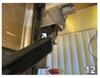
12. Shim plate installation. Slide the shim plate up and inside the space between the frame rail and the baseplate end plate. Tighten the bolts onto the side of the frame rail. Do this to both sides of the vehicle.
