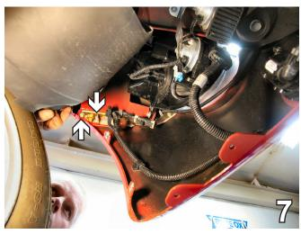
Using a 10MM socket, remove three metric bolts from underneath the fascia. Do this to both sides of the vehicle. Pull forward on the front fascia to remove. Set bolts and fascia aside to be reinstalled.
