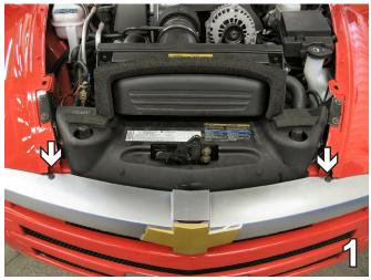
Using a 7MM socket, remove two metric bolts from silver plastic piece that rests on the top of the fascia. Pull this plastic forward and set it aside with bolts to be reinstalled later.
