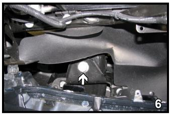
6. Remove the bolt on top of frame end, just below plastic removed in Step 4 with a 21MM socket. Reinstall the bolt with four (4) 1/2" flat washers. Do this to both sides, one side at a time.
