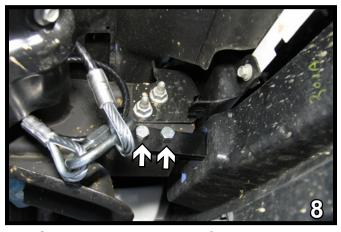
8. Slide the baseplate into frame end to align with the front tow hook hole on the outside of the frame rail. Insert straight portion of the convenience link thru the tow hook opening and align it with the existing holes of the frame. Insert a 1/2"-13 x 5" bolt, 1/2" lock washer and 1/2" lock nut into the front hole and tighten down. Do this to both sides of the vehicle.
