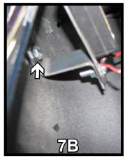
7. Remove two push pins from the opening in the grille (7A). They will be replaced with bolts and brackets (7B). Install the breakaway bracket on the passenger side with 1/4"-20 x 3/4" bolt and 1/4"-20 nut. Attach the breakaway to the bracket also with 1/4"-20 x 3/4" bolt and 1/4"-20 nut.
