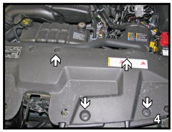
4. Remove four (4) pushpins from the flat plastic piece on top of fascia. Do this to both sides of the vehicle.
