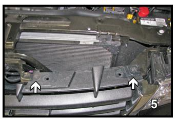
5. Using a 10MM socket remove two bolts from the top front edge of the grille. Do this to both sides of the vehicle.
