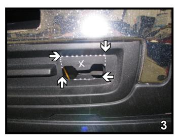
3. Using a utility knife, trim the top part of the tow hook shield. Do this to both sides of the vehicle.
