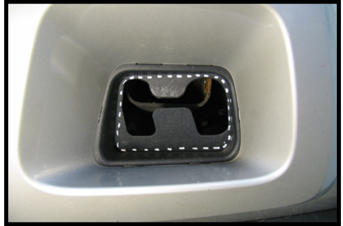
14. Hold the fascia up to the vehicle as close to its original position and mark for baseplate clearance. Trim as needed, with a utility knife, then reinstall the fascia.
