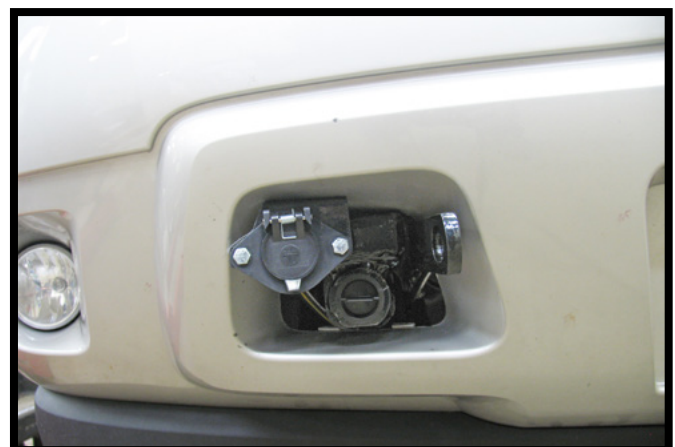
16. Possible location for the electrical bracket.
