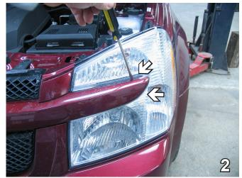
2. Insert a flat screw driver, and pop out the corner of the fascia over the headlight. Do this on both sides.
