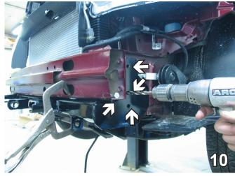
10. Using the baseplate as a template, with the 13/32" drill bit, drill all four holes on each side. Do this to both sides of the vehicle. Insert  $3/8-16 \times 2$ " hex bolts, 3/8" lock washers with Loctite Red. Attach to  $1/4 \times 1 \times 1$ " nut plates inserted into the frame and tighten. Do this to both sides of the vehicle.
