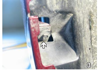
3. Using a 7MM socket, remove bolt just forward of the front tire on the wheel well. Do this to both sides of the vehicle. Set bolts aside to be reinstalled later.
