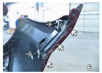
The fascia is then ready to be removed from the vehicle. Lift the corners of the fascia above the three little knobs holding the edge (white arrows). Do this on both sides. Squeeze the two push pins (gray arrows) in order to remove the fascia. Do this on both sides. Then set fascia aside carefully to be reinstalled later.
