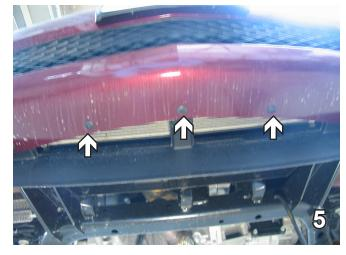
5. Using a flat screw driver, remove five push pins from the lower edge of fascia all the way around. Set push pins aside to be reinstalled later.
