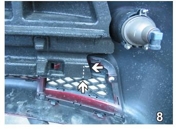
8. Using a reciprocating saw, trim away plastic area, 1" across and up, located on the back side of the fascia.
