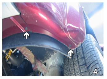
Using a 7MM socket, remove two bolts from the lower edge of fascia all the way around. Do this to both sides of the vehicle. Set bolts aside to be reinstalled later.
