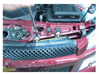
1. Using a 10MM socket, remove four bolts from the flat plastic piece on top. Do this to both sides, two on each side, of the vehicle. Set bolts aside to be reinstalled later.
