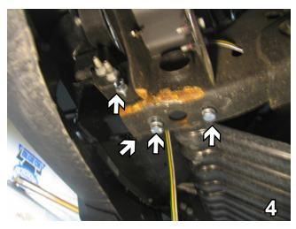
Start all four bolts, remount any hole if necessary as every vehicle is different. Insert 1/2 x 1 1/4" hex bolts with 1/2" lock washers. Be sure to use Loctite Red on all bolts. Do this on both sides.
