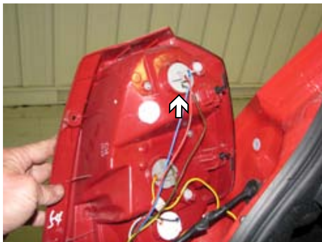
Possible location of the Bulb and Socket Wiring Kit (BX8869)
