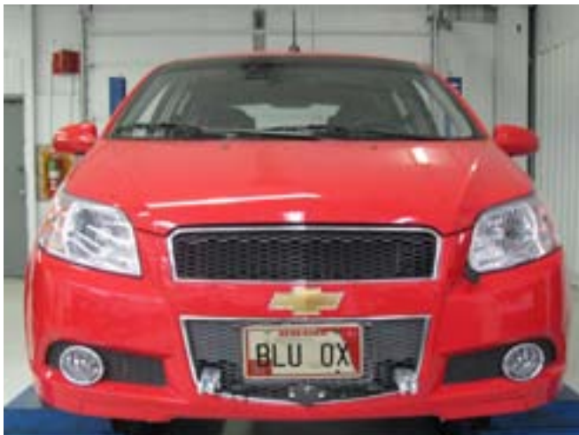
Shown with removable tabs installed.
