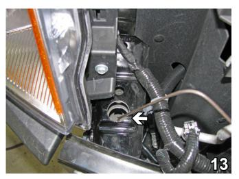
13. On the passenger side, on top where the wires have been removed, using a 1-1/4" hole saw, drill an access hole through two (2) layers.
