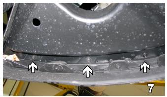
7. Using a 7MM socket, remove twelve (12) bolts across the bottom of the belly pan.
