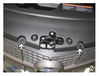
2. Remove the push pins from the center of the front.
