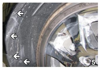
5. Using a Phillips screwdriver, remove four (4) screws just forward of the front tire on the edge of the wheel well. Do this to both sides of the vehicle.
