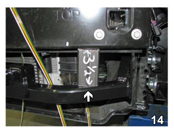
14. Position the baseplate onto the vehicle. Leaving a 3-1/2" gap from the bottom of the bumper to the top of the crosstube of the baseplate. Level and securely clamp the baseplate to the frame.
