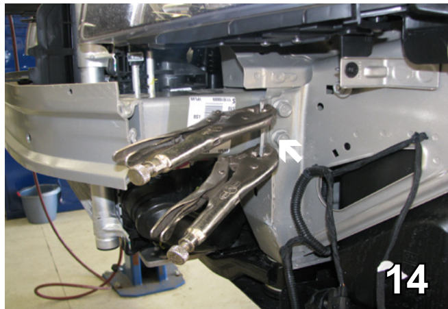
14. Using vice grips, bend the metal edge over and flatten with a hammer. Do this on both sides.
