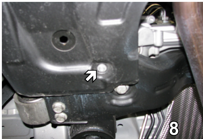
8. Using an 8MM socket, remove one more metric bolt toward the back of the belly pan. Do this on both sides. Set bolt aside to be reinstalled later.
