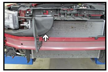
8. Remove the air baffle from the passenger side, disconnecting it from the connection by the wheel well.
