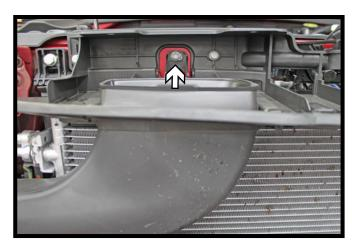
On the passenger side using a 10MM socket, remove the bolt from the top of the air baffle.
