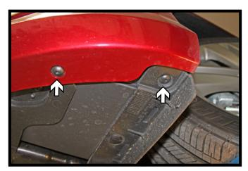
3. Using a T20 torx, remove the two (2) screws from the underside of the fascia. Do this on both sides of the vehicle.
