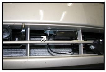
22. **Optional:** Attach the breakaway bracket to the bottom of the bumper between two fascia ribs with two 10-16 x 1" self drilling screws. Attach the breakaway to the bracket with a 1/4" x 3/4" bolt and nut.
