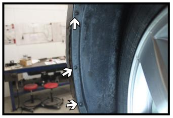
Using a T20 torx, remove the three (3) screws from the edge of the wheel well. Do this on both sides of the vehicle.
