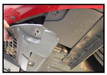
In front of the front tire, pull the lower air dam off the pin. Then pull the lower shield off the pin also in order to remove the fascia.
