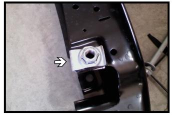
9. Remove the factory nut bracket from the bumper. Do this on both sides of the bumper.
