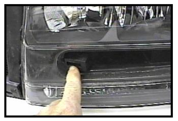
2. **Trailblazer Only:** The grille is also attached towards the middle of the headlight assembly. Pull forward to release the clip. Do this on both sides of the vehicle and set the grille aside.
