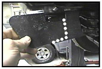
10. Trim the shrouding on both sides of the vehicle as shown.
