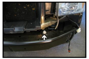
Using a 21MM socket, remove the two (2) bolts from the top of the bumper. There is one (1) on each side. Remove the bumper from the vehicle.
