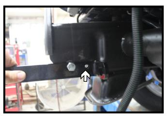
9. Place the convenience link against the frame and pin the front hole with a 1/2" bolt. Level the link and mark the frame for the rear hole. Do this on the inside passenger and outside driver frame rails. Using a 1/2" drill bit, drill out both holes to line up with the existing holes on the other side of the frame.
