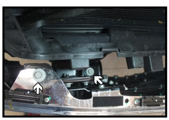
5. Using a 18MM socket, remove the four (4) bolts from the top of the bumper. There are two (2) on each side.
