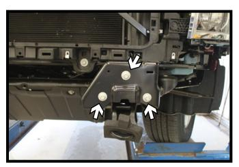
Using a 15MM socket, remove the three
