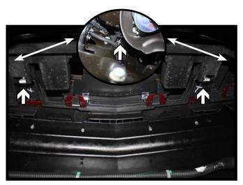
Using a 10MM socket, remove the four (4) screws from the underside of the fascia.
