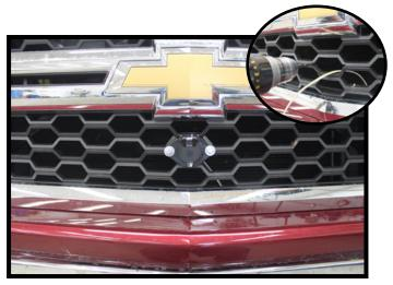
13. **Optional:** Prior to fully reinstalling the fascia. Using a 1/4" drill bit, widen the grille opening to accomodate the plug bolts. Using 1/4" x 1-1/2" bolts with 1/4" washers, install the plug thru the grille. On the backside of the grille, install the electrical bracket and 1/4" locknuts to secure the plug to the grille.
