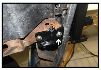
4. Install a 1/2"-13 x 1-3/4" bolt with 1/2" lock and flat washers into the front hole and a 1/2"-13 whiz nut on the inside of the frame. Do this on both sides of the vehicle. Fully tighten all hardware.
