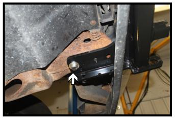
3. Position the baseplate onto the frame, aligning to the holes in the frame and clamp in place. Install a 1/2"-13 x 1-3/4" bolt with 1/2" lock and flat washers into the rear hole and a 1/2"-13 nut plate on the inside of the frame. Do this on both sides of the vehicle. Fully tighten all hardware.
