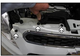
1. Remove the six (6) push pins from along the top edge of the fascia. There are three (3) on each side.
