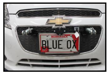
14. Hold the fascia as close to its original position, mark and trim the fascia around the convenience links and attachment tabs. Reinstall the fascia.
