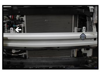
Bend the passenger side bumper tab back slightly for baseplate clearance (white).
