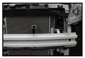
13. Optional Breakaway: Install the bracket to the bumper with the 1/4" hardware approximately 16" from the end on the driver side or in the desired location. Install the breakaway to the bracket with the 1/4" hardware.
