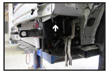
13. Using a 3/8" drill bit, drill the top front hole. Install 3/8" hardware. Do this on both sides of the vehicle. Remove vise grips.
