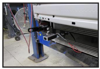
20. **Optional Breakaway:** Attach the breakaway switch to the bracket on the passenger side of the vehicle using the 1/4" hardware.
