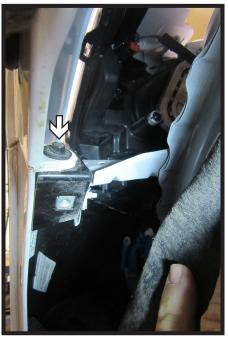
4. Pull back the wheel well liner. Using a 7MM socket, remove the one (1) bolt at the fascia joint. Do this on both sides of the vehicle.
