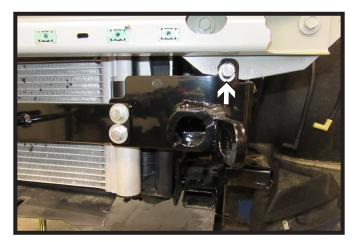
17. Using a 3/8" drill bit, drill the one (1) hole on the front of the bumper. Install 3/8" hardware. Do this on both sides of the vehicle.
