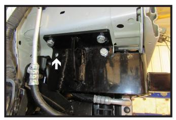
16. Using a 3/8" drill bit, drill the one (1) back hole. Install 3/8" hardware. Do this on both sides of the vehicle.
