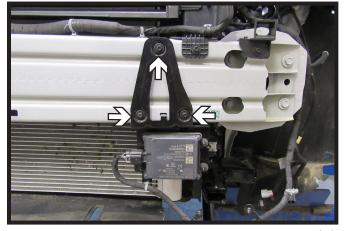
Using a 7MM socket, remove the three (3) bolts from the ACC bracket on the driver side of the vehicle. Remove bracket and set aside to be reinstalled later.
