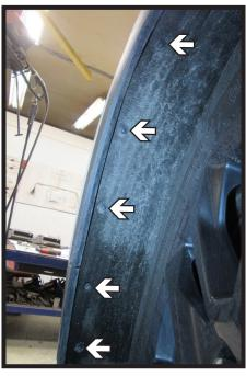
3. Using a T15 Torx, remove the five (5) bolts along the edge of the wheel well. Do this on both sides of the vehicle.
