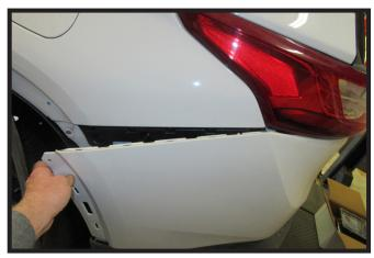
4. Grab the rear panel behind the tire and pull away from the vehicle all the way under the tail light. Do not fully remove panel. Remove tail light and install tail light wiring kit. Once installation is complete, reinstall all items. Do this on both sides of the vehicle.
