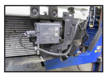
8. Unsnap the ACC wire loom from the shutter housing and bumper on the driver side of the vehicle.
