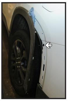
2. Grab the wheel well trim behind the rear tire and pop out the trim past the side and rear panel joint. Keep trim propped away from panels. Then using a 7MM socket remove the one (1) bolt under the trim. Do this on both sides of the vehicle.
