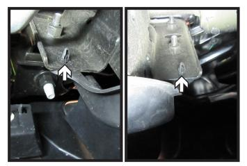
2. Remove the two (2) push pins from the rubber piece, there is one (1) on each side of the tow hook housing. Remove rubber piece, it will not be reinstalled. Do this on both sides of the vehicle.
