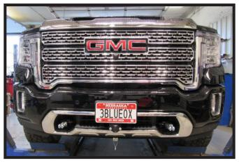
10. Attach electrical bracket and optional breakaway bracket to fascia in desired location.
