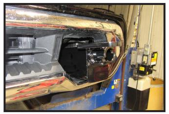
5. Tip the baseplate up slightly and slide it into the tow hook housing. Do this on both sides of the vehicle.
