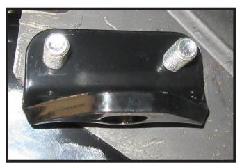
Slide the convenience link bracket onto the two (2) 1/2" bolts and place a nylon lock nut on each bolt to secure. Do this on both sides of the vehicle.
