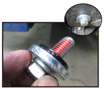
Start the one (1) 1/2" x 1-1/2" bolt with sleeve and hardware into the bottom hole. Do this on both sides of the vehicle.
