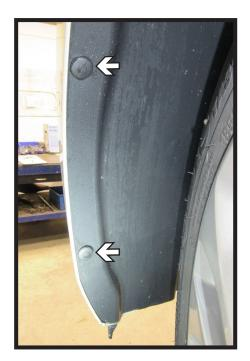
2. Remove the two (2) push pins from along the edge of the wheel well. Do this on both sides of the vehicle.
