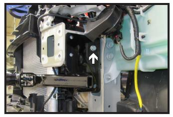
9. Slide the baseplate onto the vehicle and install a 3/8" bolt with hardware into the back hole. Do this on both sides of the vehicle.
