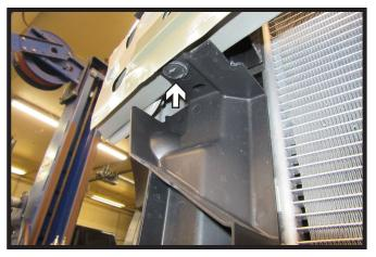
5. Remove the four (4) push pins from the top of the bumper and two (2) from the bottom of the bumper, one (1) on each side.
