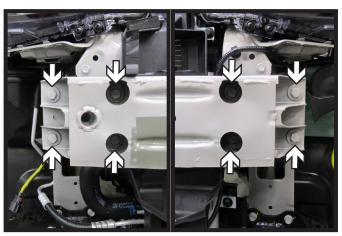
Using a 13MM socket, remove the eight (8) bolts from the bumper. Remove bumper and set aside to be reinstalled later.
