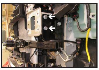
11. Install the two (2) 3/8" bolts with hardware. Do this on both sides of the vehicle.
