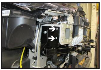
10. Using a 3/8" drill bit, drill the remaining two(2) holes using the baseplate as a guide.Do this on both sides of the vehicle.
