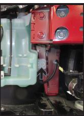
6. Remove the push pin (white) from the top of the windshield washer fluid reservoir on the passenger side of the vehicle. Then using a 10MM socket, remove the two (2) nuts (gray) and one (1) bolt (black) from the reservoir. Plug all lines, remove reservoir, and set aside to be reinstalled later.
