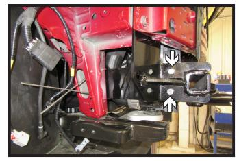
14. Attach support plate to baseplate using two (2) 3/8" x 1-1/4" bolts with hardware. Do this on both sides of the vehicle.
