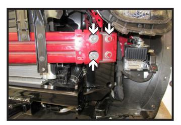
13. Install the remaining three (3) existing 10MM bolts on each side of the vehicle. Then remove starter bolt from each side and apply Locitie® Red and reinstall.
