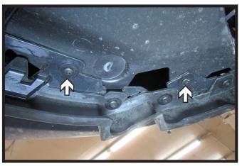
4. Using a T15 Torx, remove the four (4) bolts from the underside of the fascia in front of the tire. There are two (2) bolts on each side of the vehicle.
