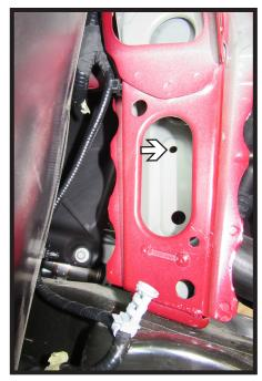
9. Using a 1/2" drill bit, drill out the top hole on the passenger side of the vehicle.
