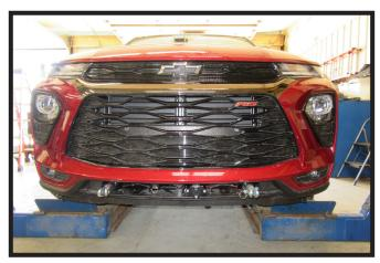
19. Hold the fascia as close to its original position, mark and trim the fascia around the convenience links and attachment tabs. Reinstall the belly pan and fascia.
