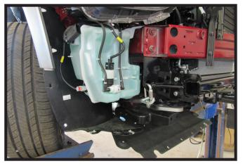
18. Reinstall windshield washer fluid reservoir on passenger side of the vehicle.
