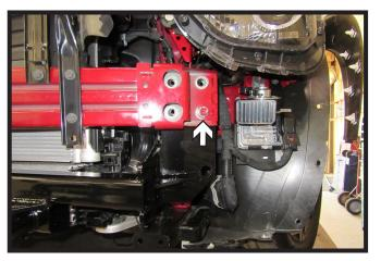
12. Slide the baseplate between the bumper and the frame. Start one (1) existing bolt on each side of the vehicle to hold baseplate in place.
