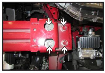
Using a 15MM socket, remove the four (4) bolts from the front of the bumper. Do this on both sides of the vehicle. Let bumper hang.
